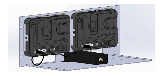
Re-install SSD caddy as before and connect cable to shogun CONNECT.
