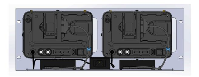
Install cable tie to secure SSD caddy extension cable.
